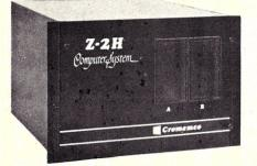
• Full 11-megabyte hard disk system • fast Z80A 4 MHz processor • two floppy disk drives • 64K RAM memory • RS232 special interface • printer interface • extensive software available List \$9995 ... OUR PRICE ONLY **\$8489**
